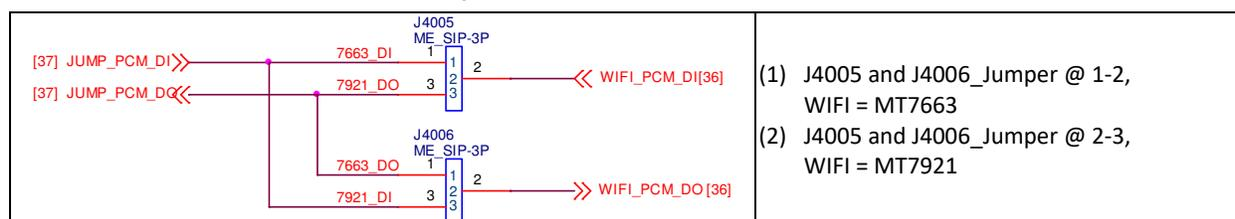
Figure 3-8. MT7921 SDIO and MT7663 SDIO Jumper Setting
