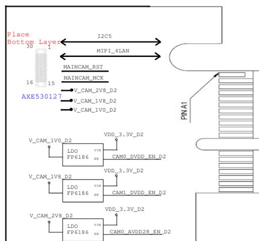
Figure 4-3. Block Diagram of D2 Camera Board
