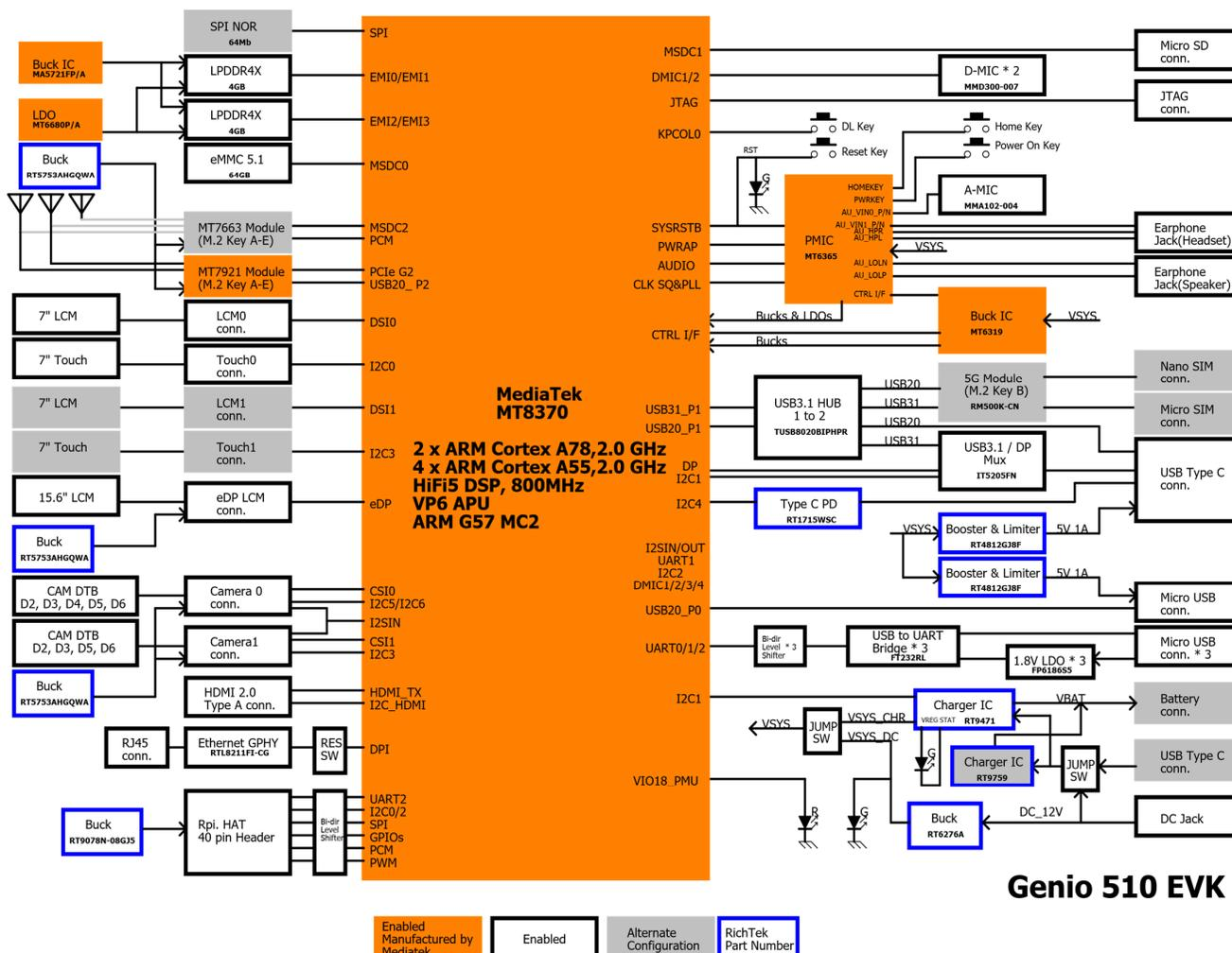
Figure 1-1. Genio 510 Evaluation Kit System Block Diagram
